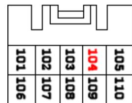
3. Cut the Black wire connecting to pin 104 of the engine ECU, leaving enough wire protruding from the connector to splice to the **long** Orange wire.
